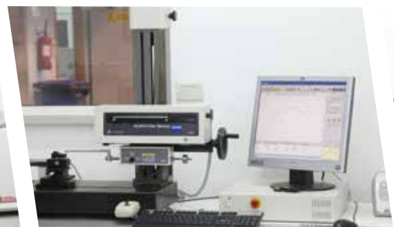
Rugosimetro/profilometro ZEISS TSK srfcom 1800 D-23-N CNC
